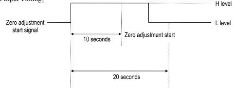
\* The start signal must be set to H level first, then it must go to L level after the passage of more than 10 seconds but not more than 20 seconds, as shown above. If the signal does not go to L level within this specified period, it will be ignored.
